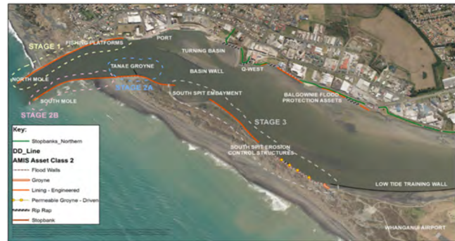
Figure 20: Te Pūwaha project stages and assets overview.
