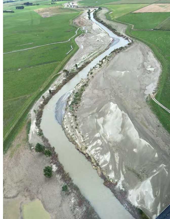
Figure 9: Ōroua River downstream of Kopane Bridge showing silt build up after Cyclone Gabrielle. The silt build up will have reduced the flood protection levels provided by the stopbanks.
